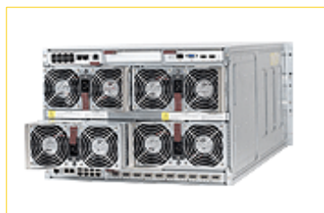
Source: Supermicro SuperBlade 3+1 redundant power supply modules
